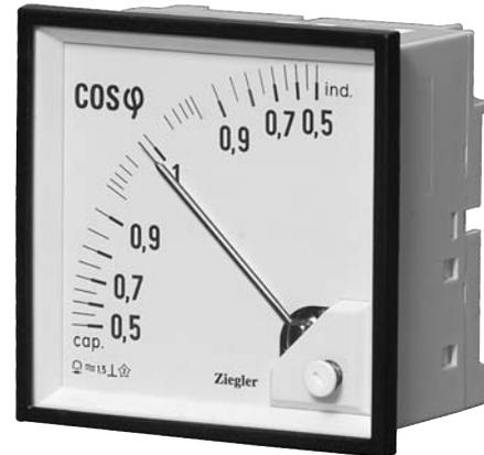
Power factor meter consist moving coil indicator with built-in SMD transducer to indicate power factor values in Single phase and Three phase systems. They come in standard size of 72x72, 96x96 & 144x144mm
