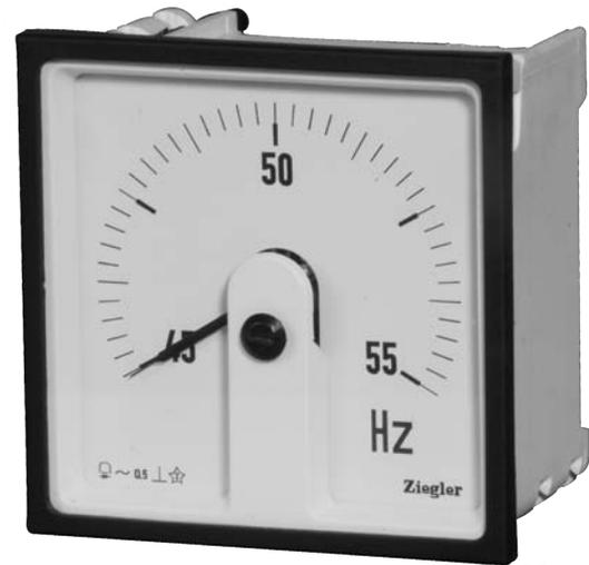
Pointer type frequency meter measure frequencies in the range of 45Hz-450Hz. For maximizing the accuracy, the essential measuring range is obtained by suppressing the unwanted frequency span. They come in standard size of 96x96 & 144x144mm
