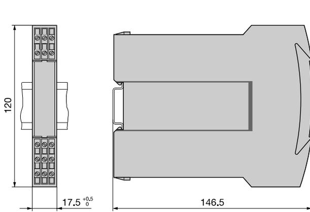
PT 602 in housing S 17 clipped onto a top-hat rail (35 X 15 mm or 35 X 7.5 mm, acc. to EN 50 022 ).
