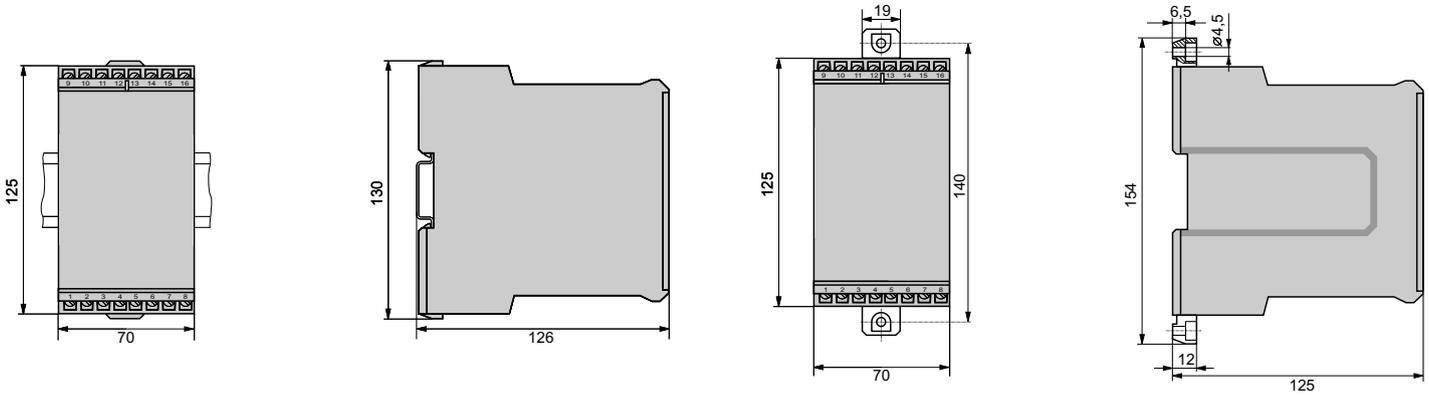
P11 in housing E16 clipped onto a top hat rail (35 x 15 mm or 35 x 7.5 mm, acc. to EN 50 022).
