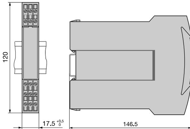
TI807-1/TV 808 in housing S 17 clipped onto a top-hat rail (35 x 15 mm or 35 x 7.5 mm, acc to EN 50 022).
