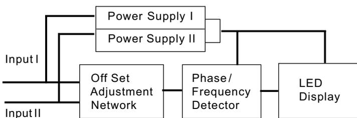
The Bus & Gen inputs are fed to the Frequency & Phase detection network. The output duty cycle of the network corresponds to the frequency difference between Bus & Generator Voltage. The detector network also determines the actual phase difference.
