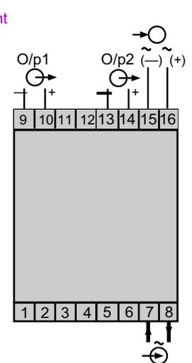
Ziegler Transducer E15 two output for AC voltage measurement.
