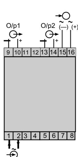
Ziegler Transducer E15 two output for AC current measurement.
