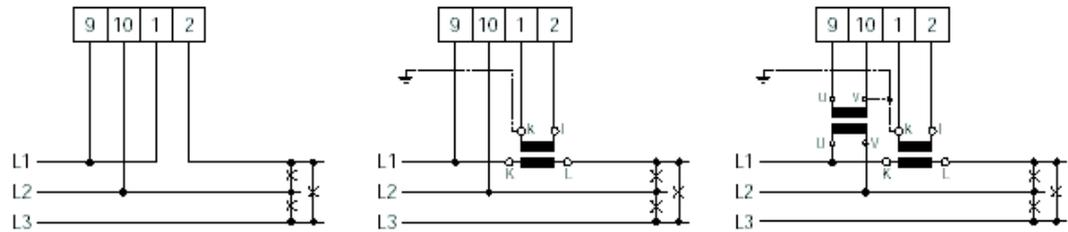
Active or reactive power measurement in 3-wire 3-phase network unbalanced load
