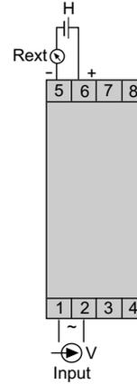
Ziegler Transducer V11, as 2-wire converter with 4.. 20 mA output.
