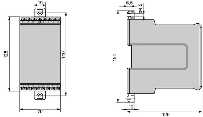
C11/C12 in housing E16 with the screw hole brackets pulled out for wall mounting.
