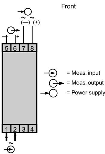
Ziegler Transducer E15 one output for AC current measurement.
