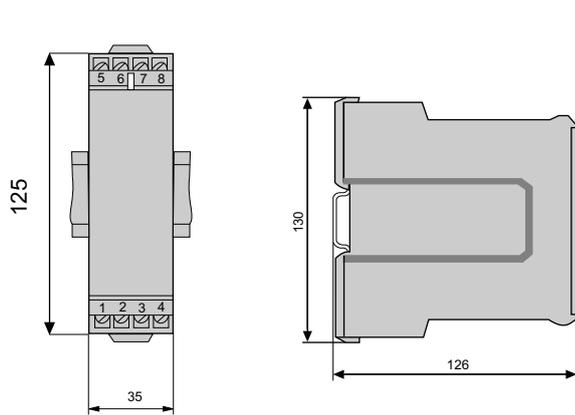
Transducer in housing E8 clipped onto a top-hat rail (35 x 15 mm or 35 x 7.5 mm acc. to EN 50 022).
