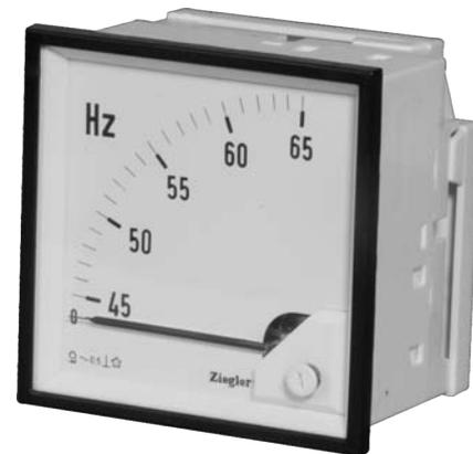
Pointer type frequency meter measure frequencies in the range of 45Hz-450Hz. For maximizing the accuracy, the essential measuring range is obtained by suppressing the unwanted frequency span. They come in standard size of 48x48, 72x72, 96x96 & 144x144mm
