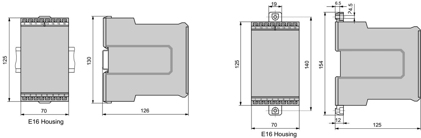
FXX in housing E8 / E16 clipped onto a top-hat rail (35 x 15 mm or 35 x 7.5 mm, acc. to EN 50 022).
