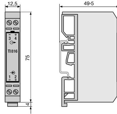
TI816 in carrying rail housing N12 on top-hat rail EN 50 022 - 35 X 7.5
