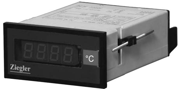
The Temperature Measuring Digital Panel Meter comes 48x96mm size. This instrument accepts resistance input from PT100 and Ni100 sensor, with 2/3/4 wire, and displays the proportionate temperature. The Temperature Measuring DPM's are designed for industrial applications which require precise and onsite adjustment for display ranges.
