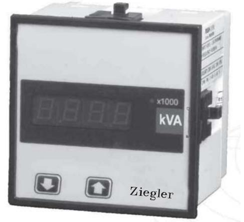
DPM 96x96 Series measures system active power (Import / Export), Reactive power(Import / Export), Apparent Power & Power Factor of three phase & single phase network. IT has 4 digit single line auto ranging LED display with polarity Indication
