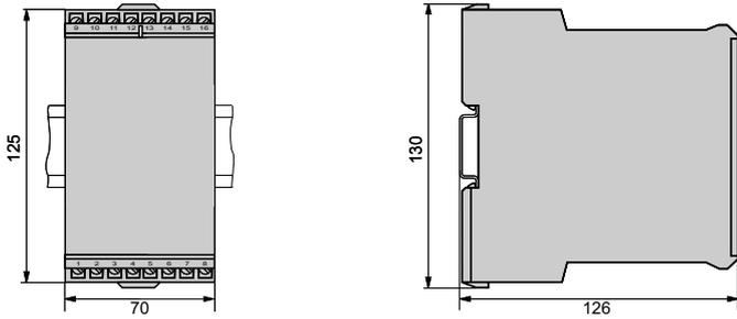
C11/C12 in housing E16 clipped onto a top hat rail (35 x15 mm or 35 x 7.5 mm, acc. to EN 50 022).
