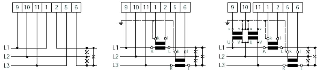
Active power measurement in 4-wire 3-phase network unbalanced load
