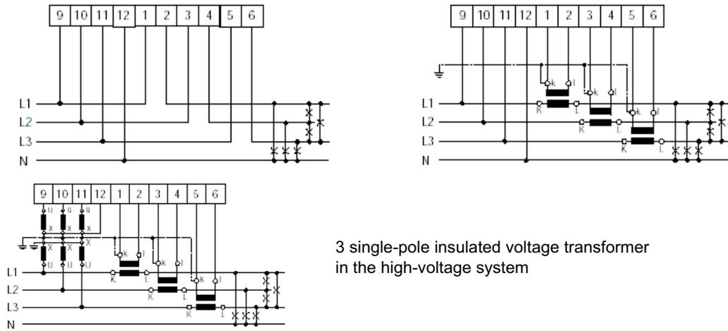
Active or reactive power measurement in 4-wire 3-phase network unbalanced load (special circuit)
