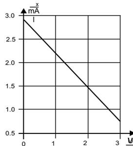
Measuring current I<sub>x</sub> as a function of the displayed voltage U<sub>x</sub> on the device under test.
