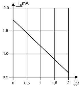
Measuring current  $I_x$  as a function of the displayed voltage  $U_x$  on the device under test.
