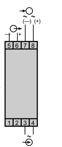
Ziegler Transducer E15 one output for AC voltage measurement.
