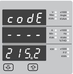
New / Change Password ,second digit entered ,prompting for third digit .(\*decimal point indicates that this will be flashing).
