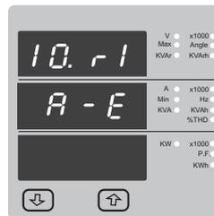
Pressing **↑** Up "key accepts the present setting and advance to" Assignment of Energy to Pulse Output 2" (see section 3.2.11).
