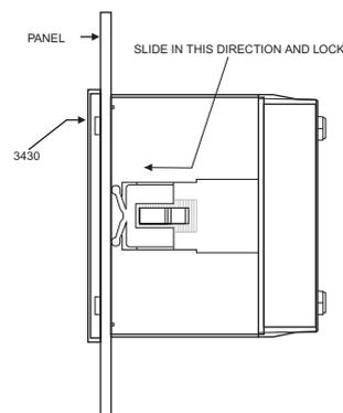
As the front of the enclosure conforms to IP54 it is protected from water spray from all directions ,additional protection to the panel may be obtained by the use of an optional panel gasket .The terminals at the rear of the product should be protected from liquids.
