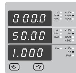
Screen 3 : System Power (Reactive, Apparent ,Active)
