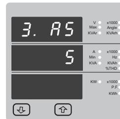
This screen is used to set the secondary value for Current Transformer .Secondary value" 5 "for 5A or "1 "for 1A can be selected .Pressing **↑** Up "key accepts the present value and advances to the Pulse Rate edit menu (See section 3.2.4) .
