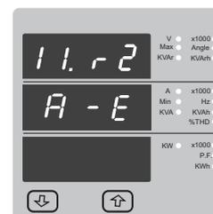
Pressing **↑** Up "key accepts the present setting and advance to" RS 485 Baud Rate)"see section 3.2.12.(
