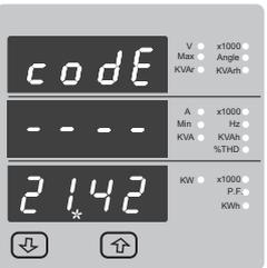
New / Change Password ,first digit entered ,prompting for second digit .(\*Decimal point indicates that this will be flashing).
