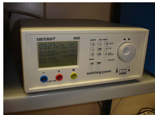
An adjustable switched-mode power supply for laboratory use
