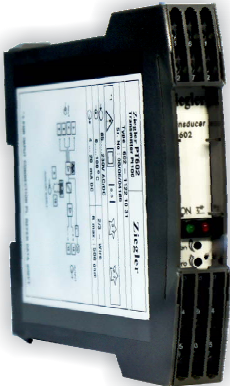
Fig. 1 .PT 602, 1 channel version, in housing S17 clipped on to a top - hat rail.
