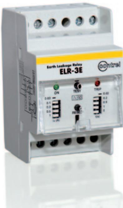
The **ELR-3E**, maintain all the basic characteristics of ELR-3C type, with reduced dimensions. It comes to complete the range of relays, built in a modular enclosure, according with DIN 43880 Standard, with a three modules width (module base 17.5 mm).
